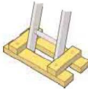
Securing at the base
